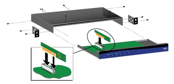
Figure 38. NetVanta VPN Accelerator Card Installation
